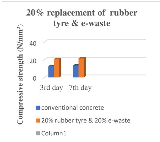
**GRAPH 2. COMPARISON OF RESULTS OF NORMAL CONCRETE 20% REPLACEMENT OF RUBBER TYRE & E-WASTE**
