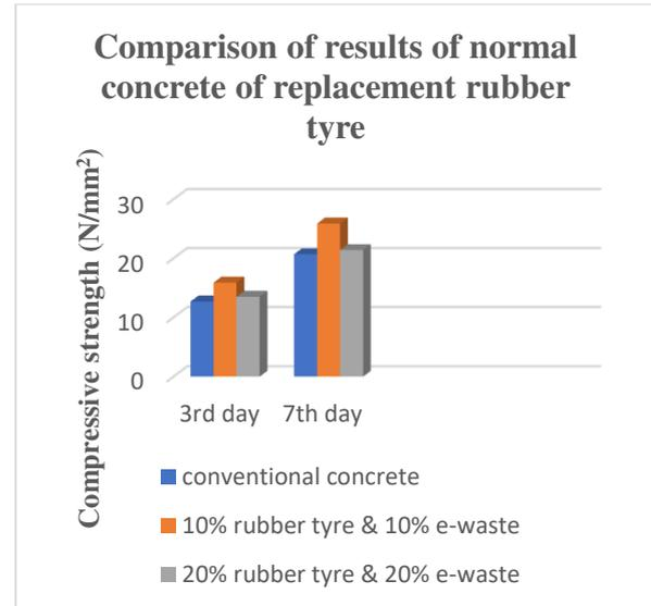
**GRAPH 3. COMPARISON OF RESULTS OF NORMAL CONCRETE OF REPLACEMENT OF RUBBER TYRE & E-WASTE**
