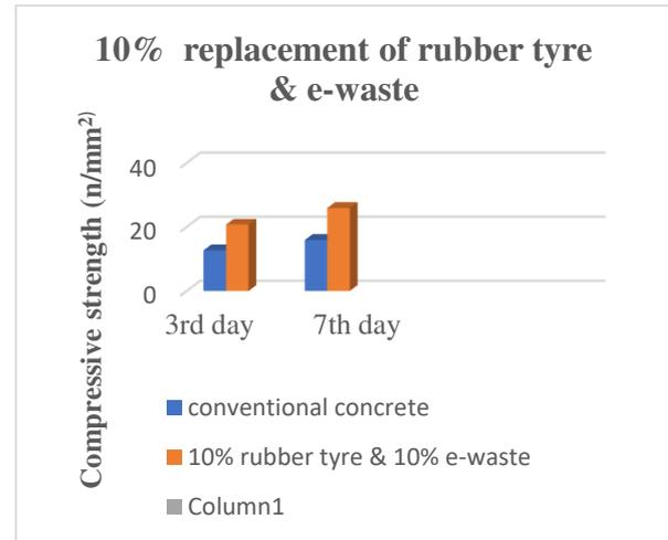
GRAPH 1. COMPARISON OF RESULTS OF NORMAL CONCRETE WITH 10% REPLACEMENT OF RUBBER TYRE & E-WASTE
